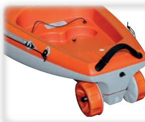
Land use configuration Wheels mounted on their axle
