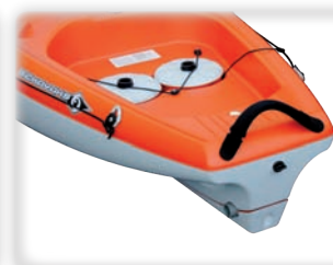
Water use configuration Wheels stowed in their storage hatch
