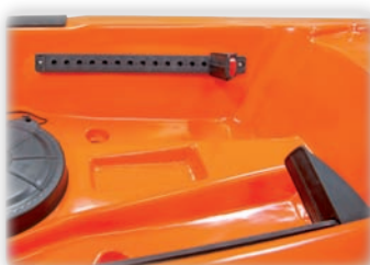
Built-in adjustable foot rests
