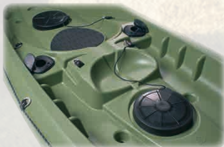
Fishing range kayaks are fitted with rod racks and watertight hatches for carrying extra equipment.
